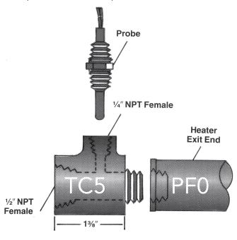
\* Thermistor adapter and catalog number TH-1 must be used for thermistor probe mounting in the TC5 fitting.
